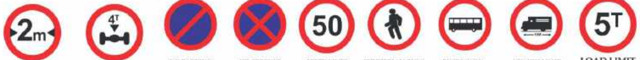
WIDTH LENGTH AXLE LOAD LIMIT NO PARKING NO STOPPING NO STANDING SPEED LIMIT PEDESTRIAN ONLY BUSES ONLY LENGTH LIMIT LOAD LIMIT
